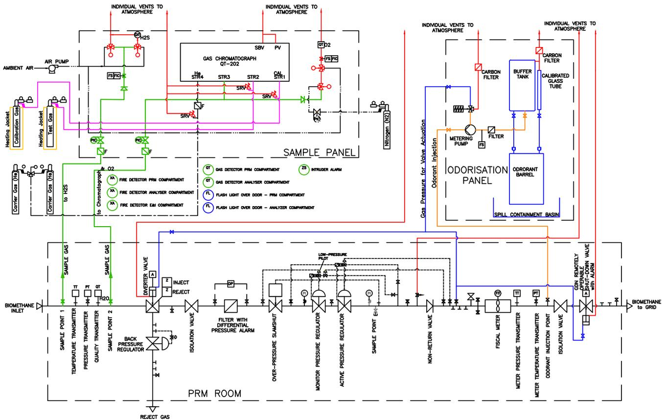
The drawing outlines details the equipment, pipework locations and the necessary valves within the BNEF.
